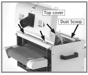
Figure 42. Top cover mounting hardware.
